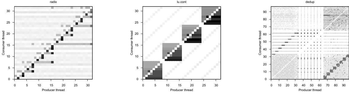
Figure 5. Spatial communication behavior: inter-thread communication during the entire parallel phase of the program for a selection of SPLASH-2 and PARSEC benchmark applications.
