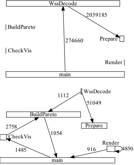
Figure 1. Communication graph after marking of the major code regions `CheckVis[ibility]`, `BuildPareto`, `WssDecode`, `Prepare[Render]` and `Render`. Region lengths (as node widths, proportional to the region's dynamic instruction count) and large inter-region communication flows (marked on each edge, in bytes) are shown, for frames #1 (top) and #2 (bottom).
