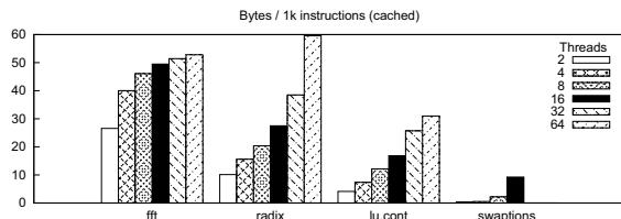
Figure 9. Inter-thread communication characterization (with perfect caching), when changing the number of threads
