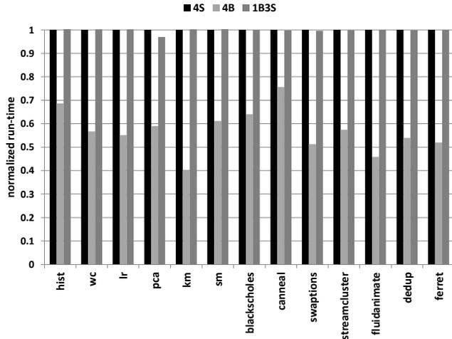
Figure 1. Normalized run-time on a homogeneous multi-core with 4 small cores (4S), 4 big cores (4B), and a heterogeneous multi-core with one big and three small cores (1B3S) while keeping threads pinned to cores.
