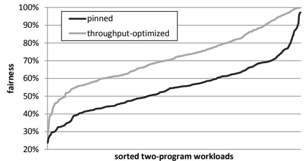
Figure 2. Fairness for a 1B1S system for pinned versus throughput-optimized scheduling using PIE for 500 randomly chosen two-job mixes.
