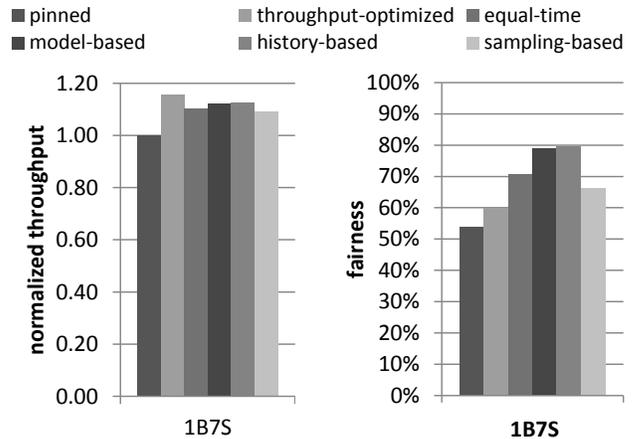
Figure 6. Evaluating different methods for estimating the big-to-small-core scaling factor in equal-progress scheduling for a 1B7S system.
