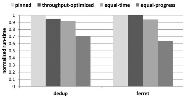
Figure 11. Comparing scheduling algorithms relative to pinned scheduling for a 1B3S system running heterogeneous multi-threaded applications.
