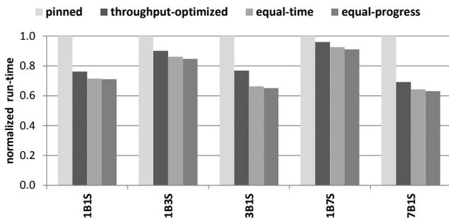
Figure 10. Fairness-aware scheduling for different heterogeneous multi-core configurations for the homogeneous multi-threaded applications.
