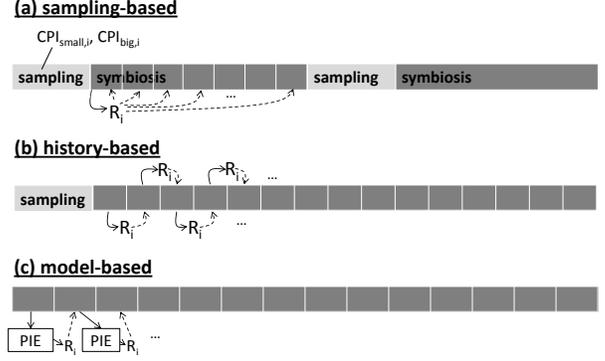
Figure 3. Equal-progress scheduling: sampling-based, history-based and model-based.
