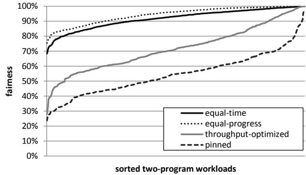
Figure 4. Comparing scheduling algorithms relative to pinned scheduling in terms of throughput (left graph) and fairness (right graph) for a 1B1S heterogeneous multi-core with one big and one small core.
