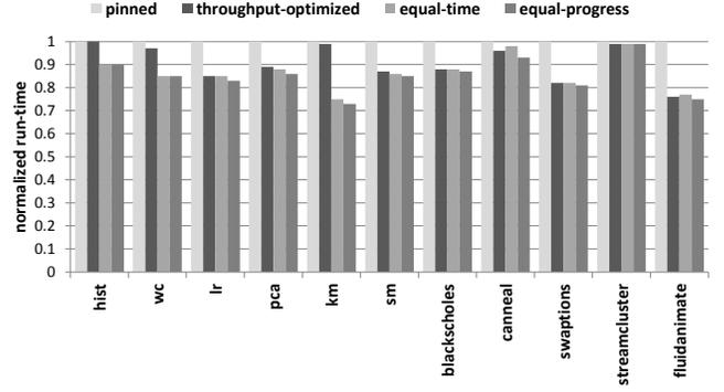
Figure 9. Comparing scheduling algorithms relative to pinned scheduling for a 1B3S system running homogeneous multi-threaded applications.
