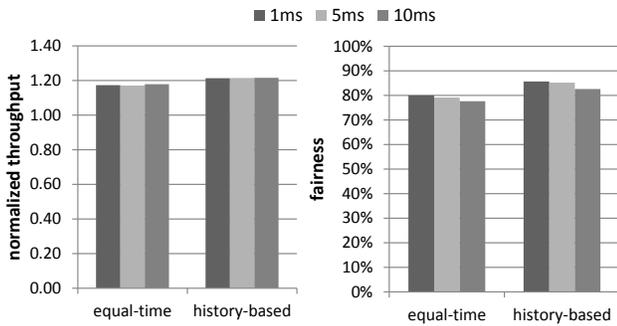
Figure 8. System throughput and fairness for equal-time and equal-progress (history-based) scheduling as a function of time slice granularity.
